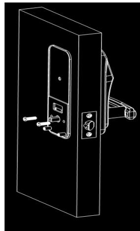
6. Fix the back iron board on the back gasket
