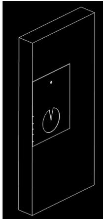
1. Determine the handle line and drill holes for with the template board.
