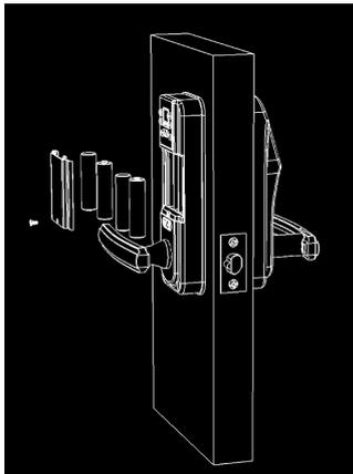
**9. Install the battery into the compartment on the back plate.**
