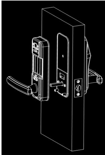
**7. Connect the cable to the back plate**
