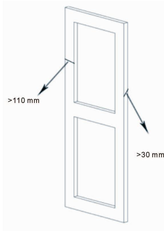
Wooden door with thickness from 30 to 60mm
