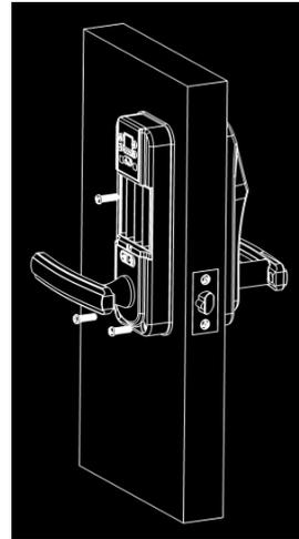
**8. Fixing the back panel with 3 screws**
