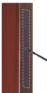
● Drill holes with depth 82-88mm
